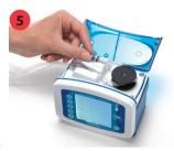
Grasp black ring retainer, and gently wrap tubing anticlockwise around rotor. Pull up retainer and insert into slot.
