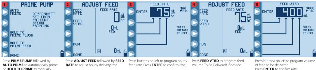
or HOLD TO PRIME to manually prime both feed and flush lines. Press **DONE** when complete.
