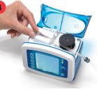
Grasp finger tab on valve and insert valve into valve slot on the left.
